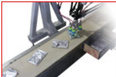
Fast and accurate pick and places are realized with the AF-DLT pick and place system. 300 pick and places per minute are achievable.
