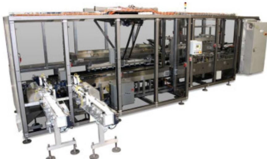
A barrel cam loading system uses a series of pushers to more smoothly move products into cartons. The HD-CMA machine can run 320 products per minute, cartoning one bag of chips per carton.
