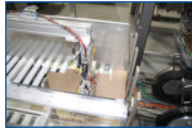
Cartesian Case Erecting eliminates tabs and pins on the magazine for fast repeatable changeover and positive wrap around case erection.
