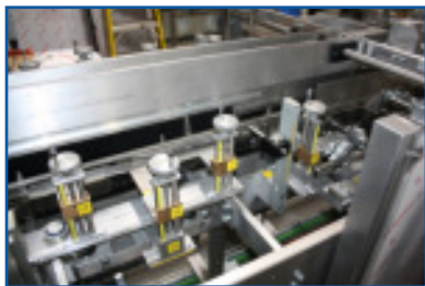
Tucking mechanism with quick change tools for fast and repeatable changeover. The HD-IMA also has the ability to run glue style cartons.
