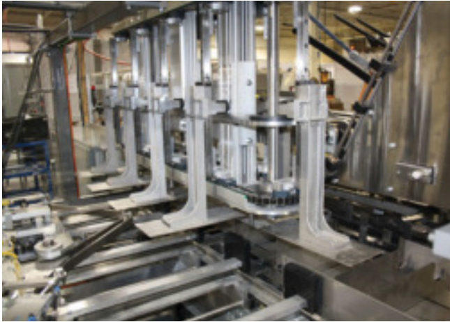
The cartoner's overhead barrel cam loader and sliding style buckets help ensure positive loading.
