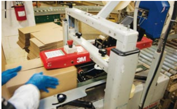
Installed on one of Johnvince Foods' stand-up pouch packaging lines, a 3M-Matic case-sealer tapes the carton shut just prior to palletizing.
