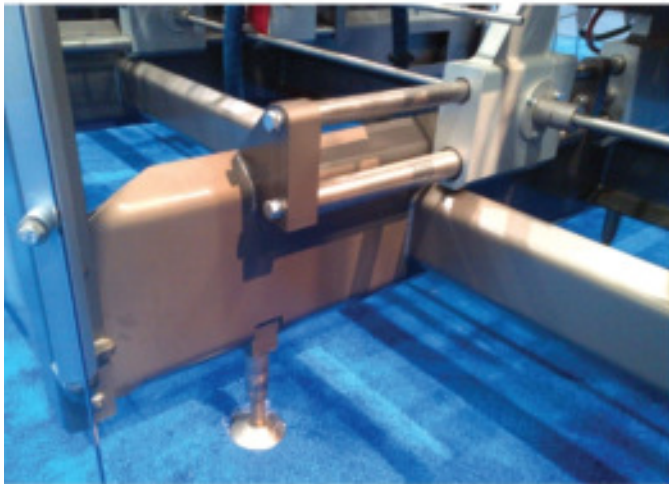
The hygienic design of the Langen C-1000H cartoner minimizes horizontal surfaces to prevent debris from collecting. The solid frame eliminates cavities that could harbor dirt and bacteria.
