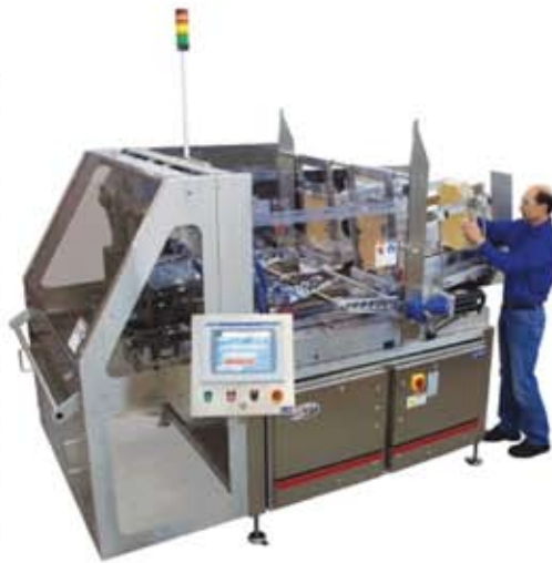
No-tool change parts on Delkor's Trayfecta forming machine cut changeover time to three minutes or less per lane. The flexible system handles cartons, trays or cases made of paperboard, microflute or corrugated. If equipped with multiple heads, the unit can produce different containers in the same cycle.
