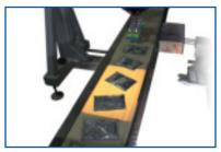
Vision System is standard on the MK-DLT pick and place system. This ensures that products do not need to come uniformly to the Delta 3 robot.
