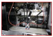
Fast and accurate pick and places are realized with the MK-DLT pick and place system. 300 pick and places per minute are achievable.
