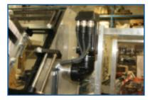
Servo drive attached to tray denestor aids in accurate feedback on positioning and fault diagnostics. In addition, the use of servo's significantly reduces the size of the tray denestor.
