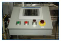
Allen Bradley control panel offers simplicity in operation and troubleshooting. In addition, the operator can effectively manage the tray denestor's speed.
