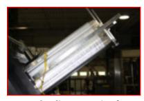
Easy loading magazine for operators. Adjustable screws on magazine allows trays to be changed over in minutes which increases productivity and lowers costs.
