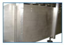
Stainless steel frame allows the tray packer to handle food applications. AFA's standard frame design ensures a rigid packaging machine and allows for easy cleaning.
