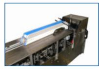
Extended magazine reduces operators time spent on refilling magazine with cartons. The extended magazine can hold up to 2'000 cartons.
