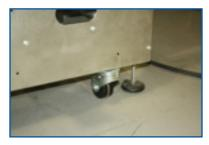
Casters allow the MK-500 to be easily moved and stored when needed. Also, casters are helpful during the integration process as no heavy machinery is needed to move the machine.
