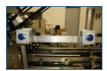
Manual load station to cycle carton. This feature improves safety for operators as the carton will not index until both hands have pushed the cycle start buttons.
