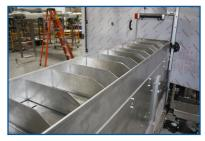
Autoload Buckets allow for semi-automated cartoning. The buckets are adjustable and AFA will provide jigs for each SKU. This allows for accurate and repeatable changeovers.
