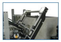
Screw adjust magazine with scales can help assist in quick and accurate changeover.
