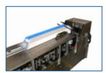
Extended magazine reduces operators time spent on refilling magazine to improve overall production. The extended magazine can hold up to 2,000 cartons.
