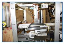
The servo driven loader can handle the most complex pack patterns. In addition, feedback on fault diagnostic and positioning accuracy are accessible with the servo loader.
