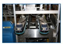
Discharge belts at the end of the MK-ISP reduce carton marking when transferring a carton onto another system. Discharge belts are also an excellent way to reduce carton jamming.
