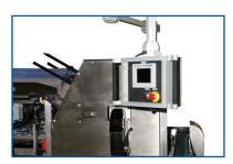
Swing arm operator panel offers an ergonomic solution for operators when troubleshooting machine faults. This feature also helps operators maintain the cartoner.
