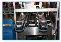
Discharge belts at the end of the TL-GDP reduce carton marking when transferring a carton onto another system. Discharge belts are also an excellent way to reduce carton jamming.
