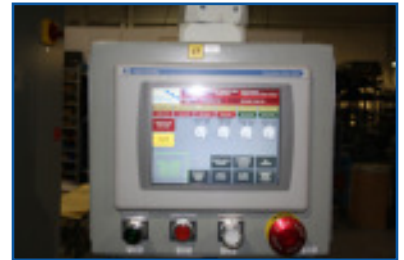
AFA's engineers can custom design the operator HMI to suit your needs. Access to servo motor set up, changeover aid, operating statistics, and more can all be included on the HMI.
