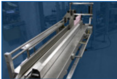
Extended Vertical Magazine is at an ergonomic level so operators can easily load the magazine. In addition, the extended magazine allows for continual operation.
