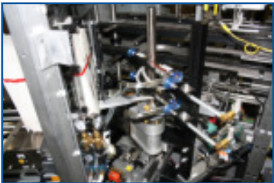
Vertical Rotary Feeder with Prebreak Mechanism is servo driven for smooth operation and provides positive feeds into the cartoner's main conveyor.
