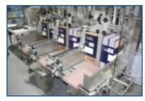
Vertical magazines are designed to ensure adequate back pressure and squaring for case/ carton erecting. Easy loading is also featured in the case/carton magazines.
