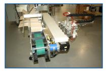
The CE-ABI index conveyor is servo driven allowing for smooth operation. Also, the auto-bottom cartons are easily picked and placed onto the discharge conveyor.
