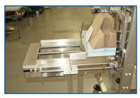
Auto-bottom carton magazine is at an ergonomic level allowing your operators to easily load the magazine. No step ladder is needed with this auto-bottom carton magazine.
