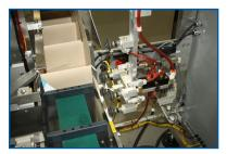
Horizontal auto-bottom carton erector can easily pick and erect auto-bottom cartons. Minimal jams are incurred when using this carton erector allowing for increased up-time.
