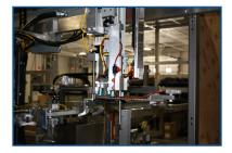
Flat Stack Magazine™ and **Cartesian Case Erecting** eliminates tabs and pins on the magazine for fast repeatable changeover with no adjustments of tabs and pins.
