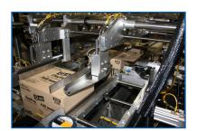
**Engineered folding and guide** rails coupled with advanced gluing technology ensures square cases with limited case rejects and jamming.
