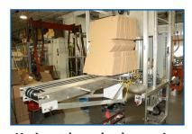
Horizontal easy load magazine is ergonomic and can hold a large volume of DSSC's. The horizontal orientation of the magazine makes loading easier and quicker for operators.
