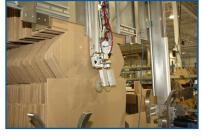
Vertical forming head allows the CF-DSS to incur a small footprint. This feature also decreases costs as no female tool is required for forming cases.
