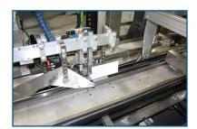
Glue or tape closure can be applied to the CS-TOP. The CS-TOP can also reach speeds of over 30 cpm with cases or cartons with AB Servo Drives and Motors.
