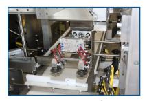
AFA can custom engineer a collating system that fits your application. In this application, a servo driven pick head stacks the cartons until the correct pack pattern is achieved.
