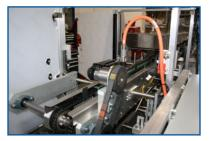
Servo Driven Overhead Squaring Chain can provide high quality closures on cartons over 2" wide. This system will allow for a square closure on your carton.
