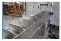
Autoload Buckets allow for semi-automated cartoning. The buckets are adjustable and AFA will provide jigs for each SKU. This allows for accurate and repeatable changeovers.
