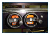
Digital scales allow operators to reference different carton and product configurations. This reduces changeover time resulting in better overall packaging efficiency.
