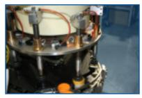
**Compact Rotary Turret can** achieve speeds greater than 300 ppm. In addition, provides easy visibility for operators during troubleshooting because of its compact size.
