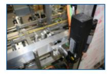
Servo Driven Tucking Mechanism ensures consistent flap closures. This Tucking Mechanism can handle speeds greater than 300 ppm.
